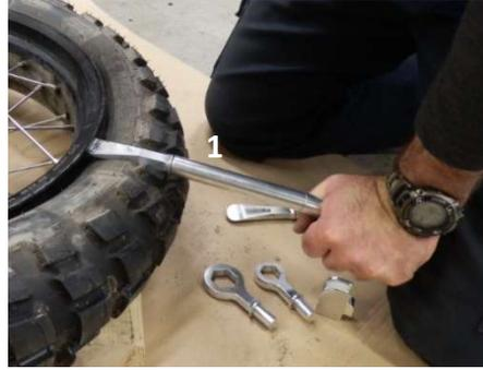
Step 2; Assemble the spoons & levers. Push spoons 1 between rim and tyre. Lever it up and down to loosen (a possibly sticky) tyre somewhat from the rim. Repeat over an area of approx. 10 inch.
