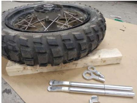
Step 1; Remove the wheel, lay it on a flat underground. Take care of sensitive parts like ABS rings and brake rotors. Don't let dirt enter the seals and bearings.
